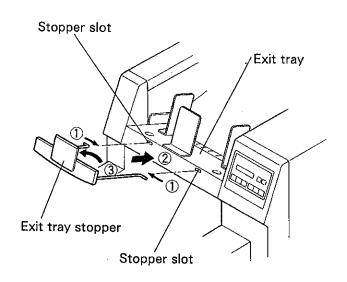
Push the ends of the exit tray stopper wires slightly together, and insert them into the stopper slots of the exit tray. Then pull up the plastic part of exit tray stopper. (Install the exit tray stopper in the sequence of ① through ③.)
