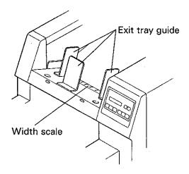
Position the exit tray guides against the document width scale. (Secure the guides in place.)
